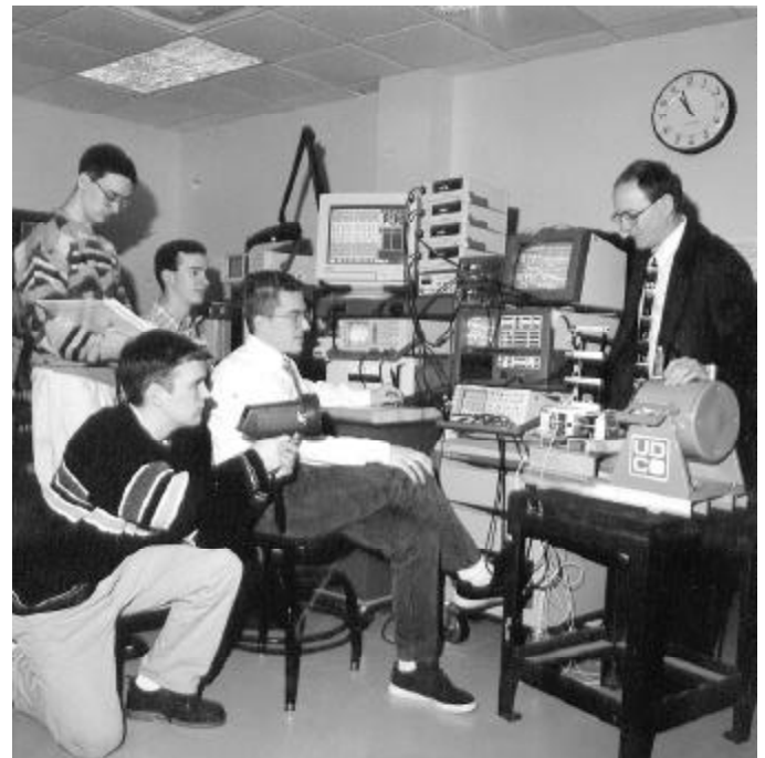
Electrical and mechanical engineering students in the vibrations course conduct an experiment on a model of a multistory building. Dr. Larry Zavodney, chairman of the Department of Engineering, observes the demonstration.
